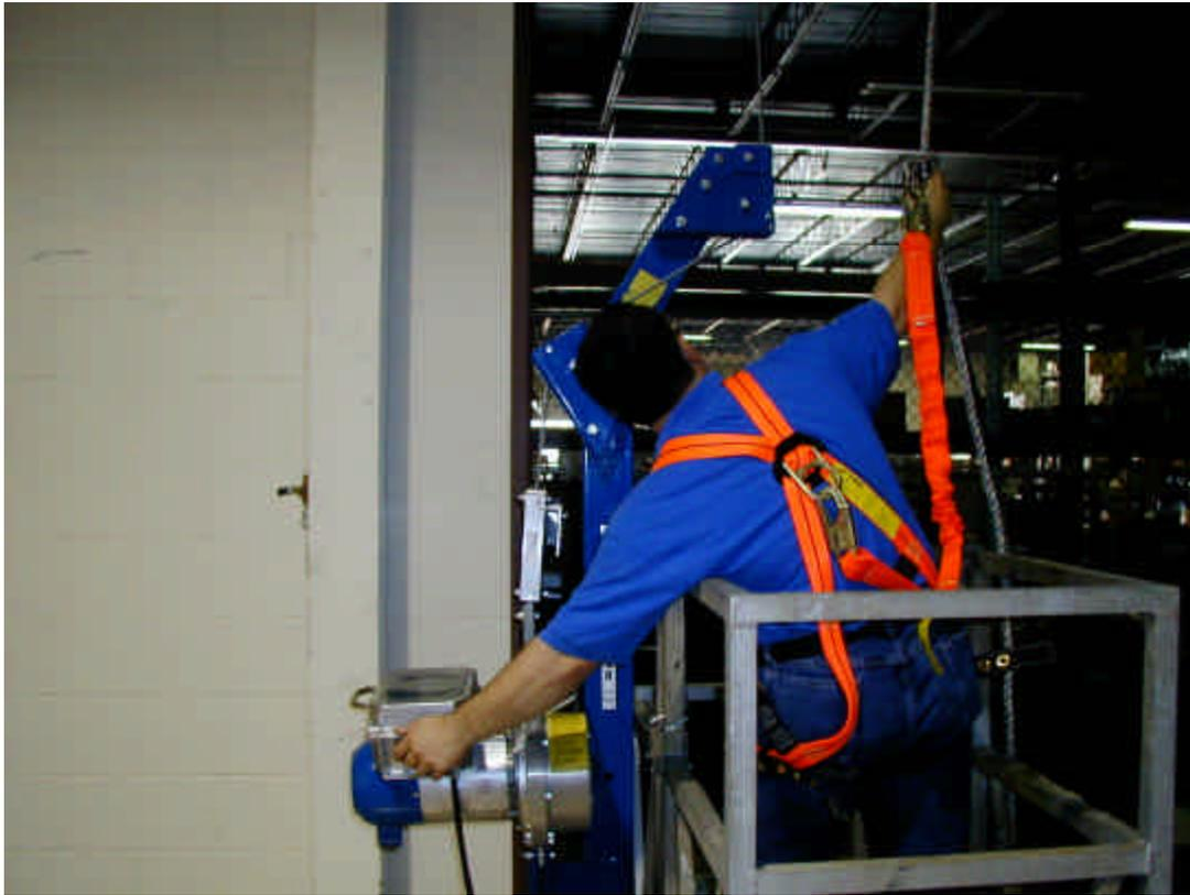
**Figure 9 - Operator using the hoist controls of Compact hoist mounted on Walk-Thru stirrup of MKD Work Cage.**
