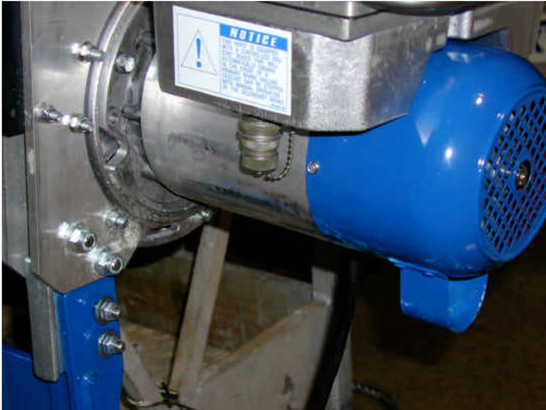
**Figure 7 - Close-up back view of Compact hoist mounted on Walk-Thru stirrup of MKD Work Cage.**
