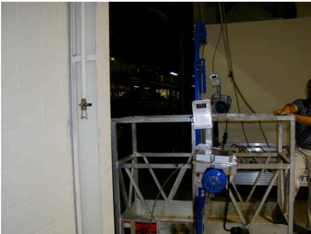
**Figure 2 - Complete side view of Compact hoist mounted on Walk-Thru stirrup of MKD Work Cage.**
