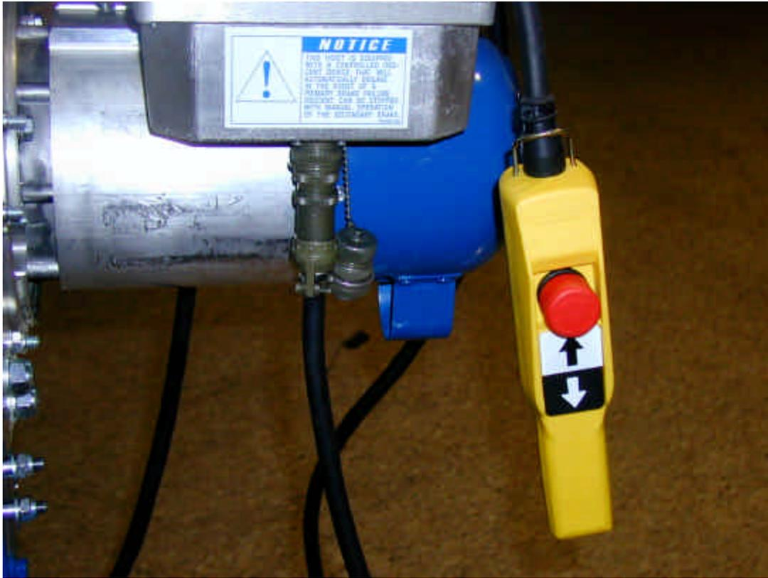
**Figure 11 - View of an optional 6-Foot Pendant Control (P/N: 41021752-6) and its connection on the Compact hoist. Pendant Control is connected by simply removing the Jumper Plug connection from back of hoist and connecting the Pendant Control connection\*. Hoist can then be operated by either the hoist mounted controls or the pendant controls.**
