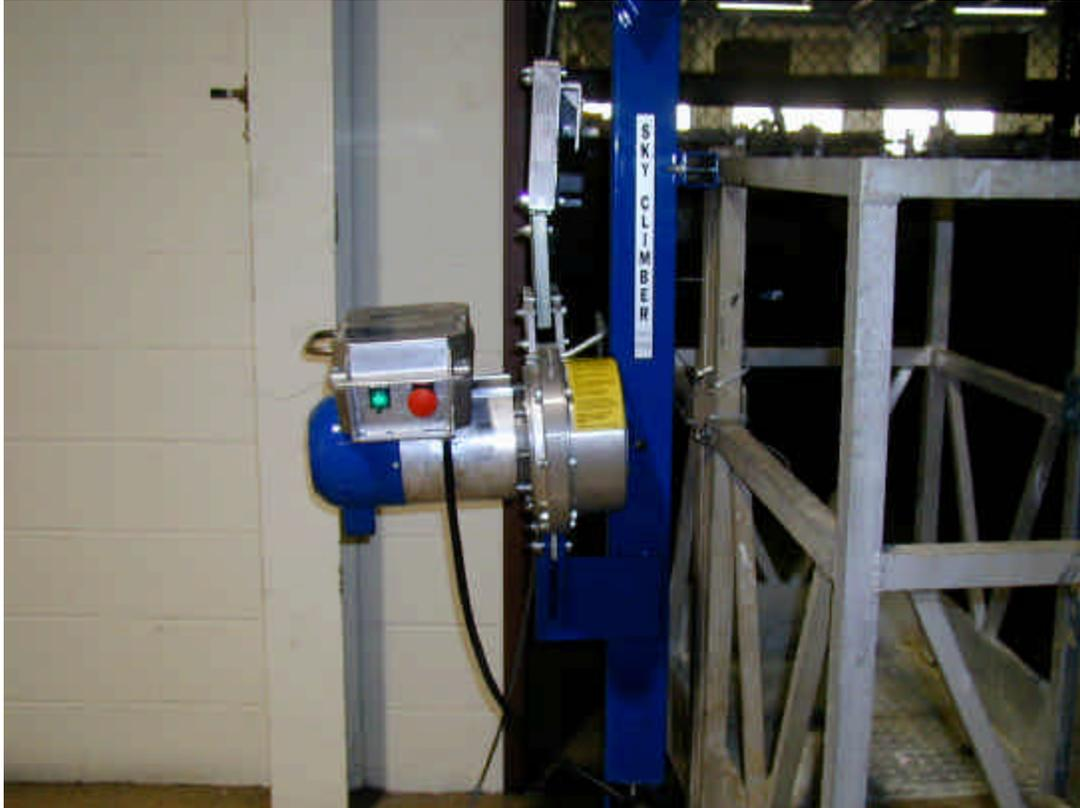
**Figure 3 - Front view of Compact hoist mounted on Walk-Thru stirrup of MKD Work Cage.**
