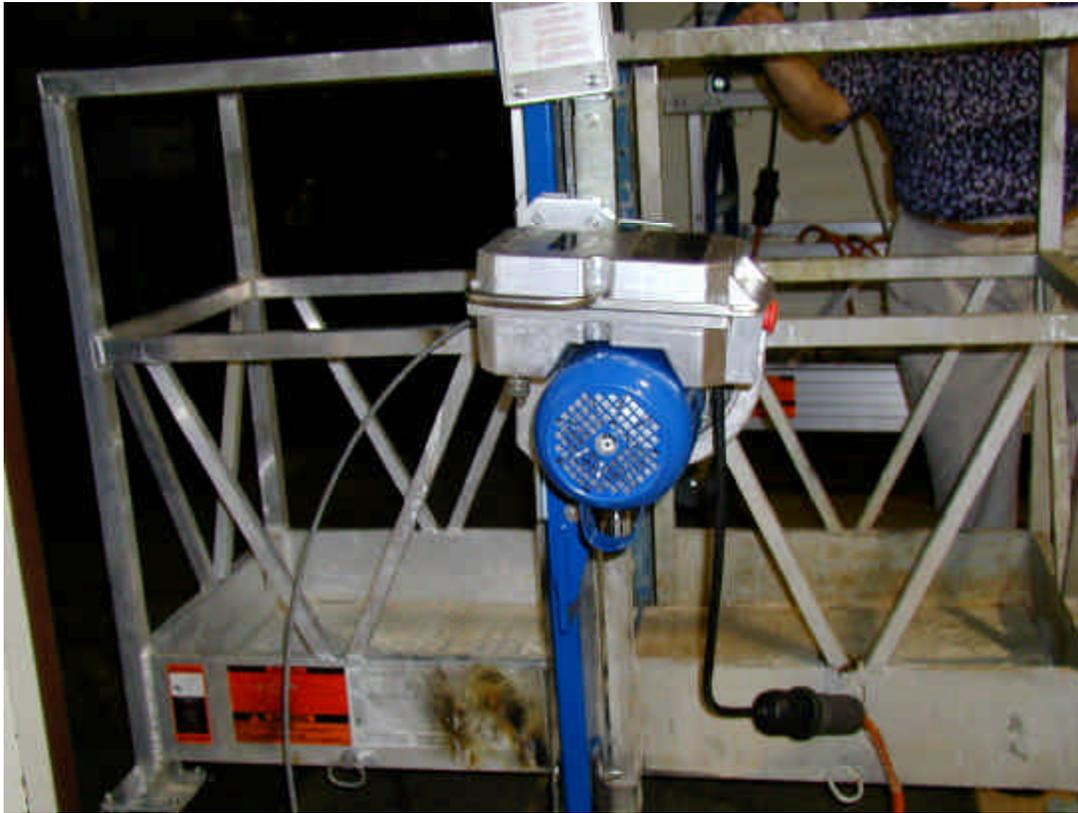
**Figure 1 - Side view of Compact hoist mounted on Walk-Thru stirrup of MKD Work Cage.**
