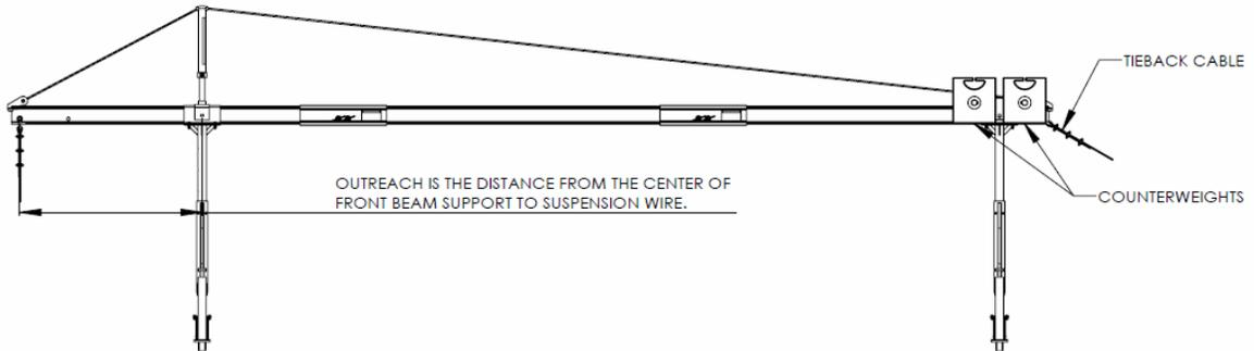
NO. OF 50LB COUNTERWEIGHTS REQUIRED PER BEAM ASSEMBLY
