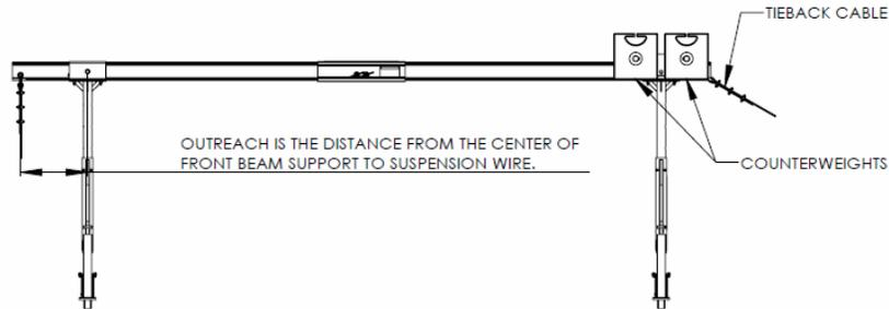
NO. OF 50LB COUNTERWEIGHTS REQUIRED PER BEAM ASSEMBLY
