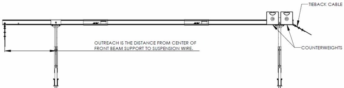
NO. OF 50LB COUNTERWEIGHTS REQUIRED PER BEAM ASSEMBLY
